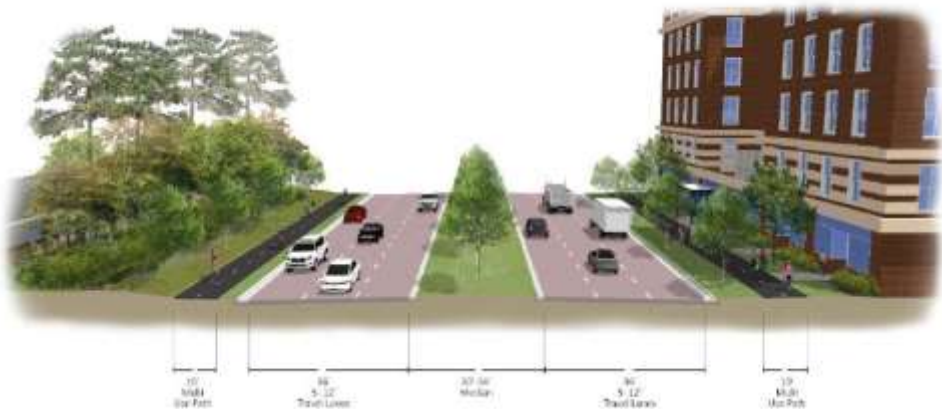
Figure 10. Six-lane synchronized street typical section
