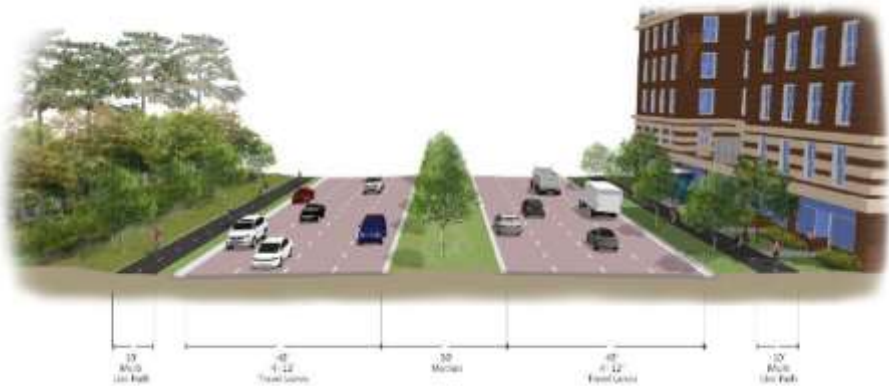
Figure 11. Eight-lane roadway typical section
