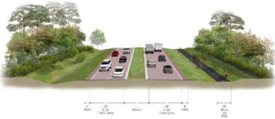
Figure 23. Four-lane divided typical section with raised median
