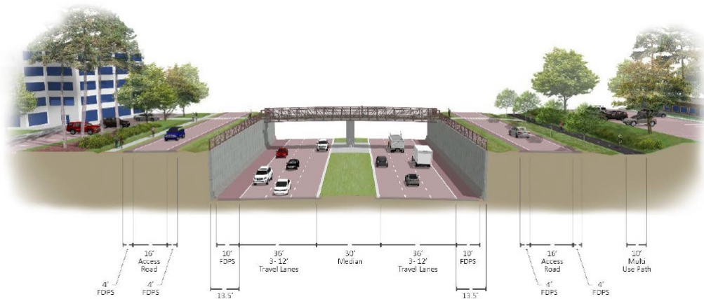
Figure 18. Six-lane depressed roadway with frontage roads typical section
