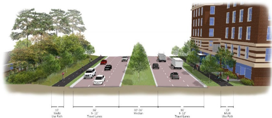
Figure 10. Six-lane synchronized street typical section
