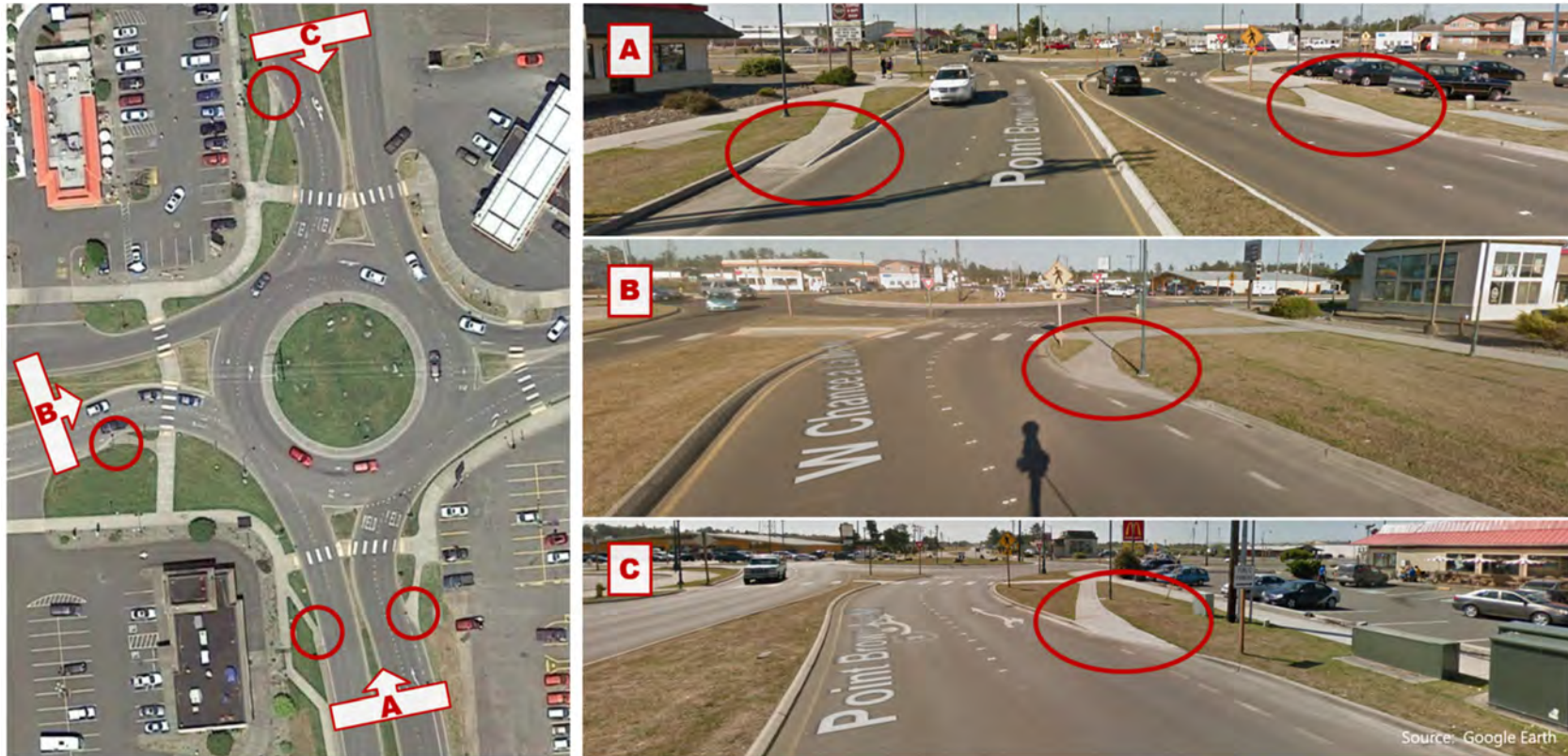
Figure 31: Example Roundabout Treatment for On-Road Bicycles
